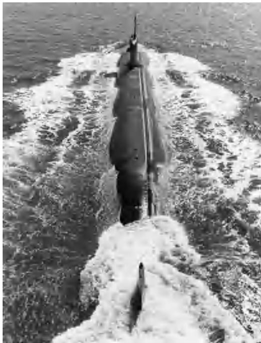
Fig. 3. Nuclear attack submarine USS *San Francisco*. The ridge running up the hull houses a towed array. (U.S. Navy)
