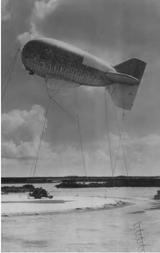
Fig. 3. Tethered balloon. (U.S. Air Force)
