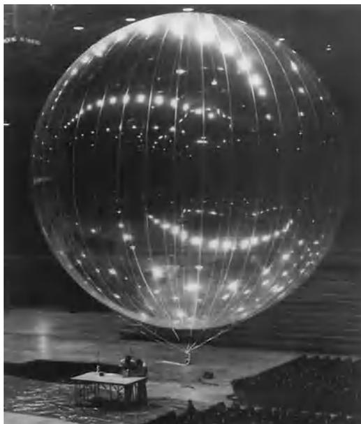
Fig. 2. Superpressure balloon. (Raven Industries)
