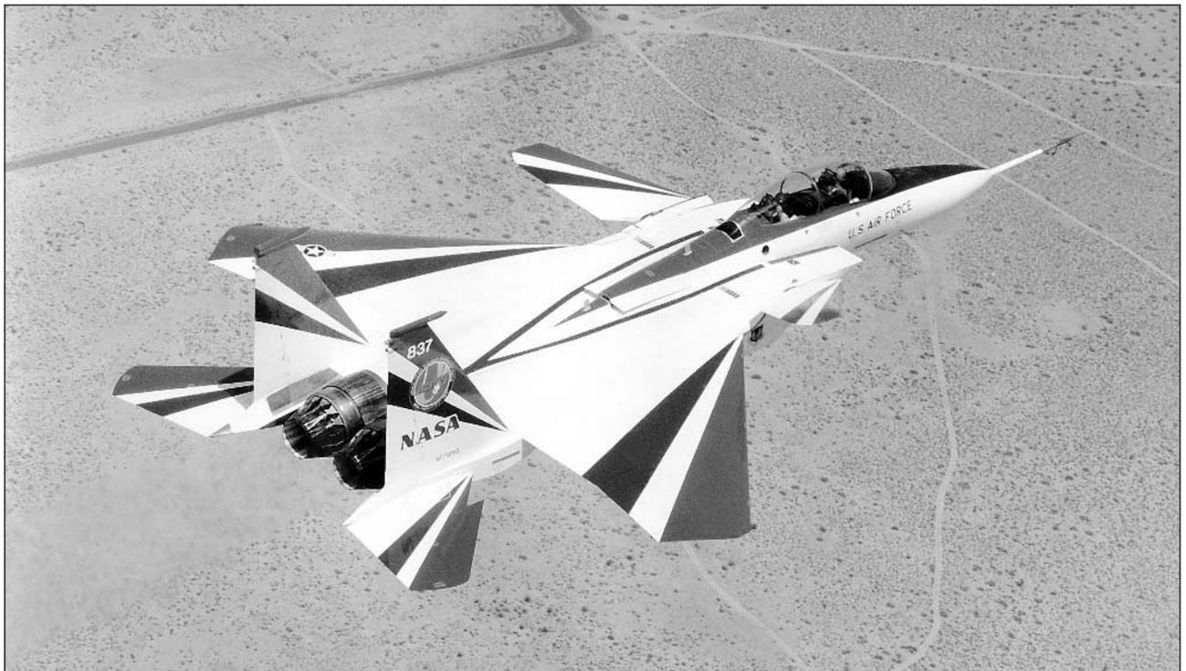
The F-15B is equipped with nozzles that allow it to control both pitch and yaw. (NASA)
