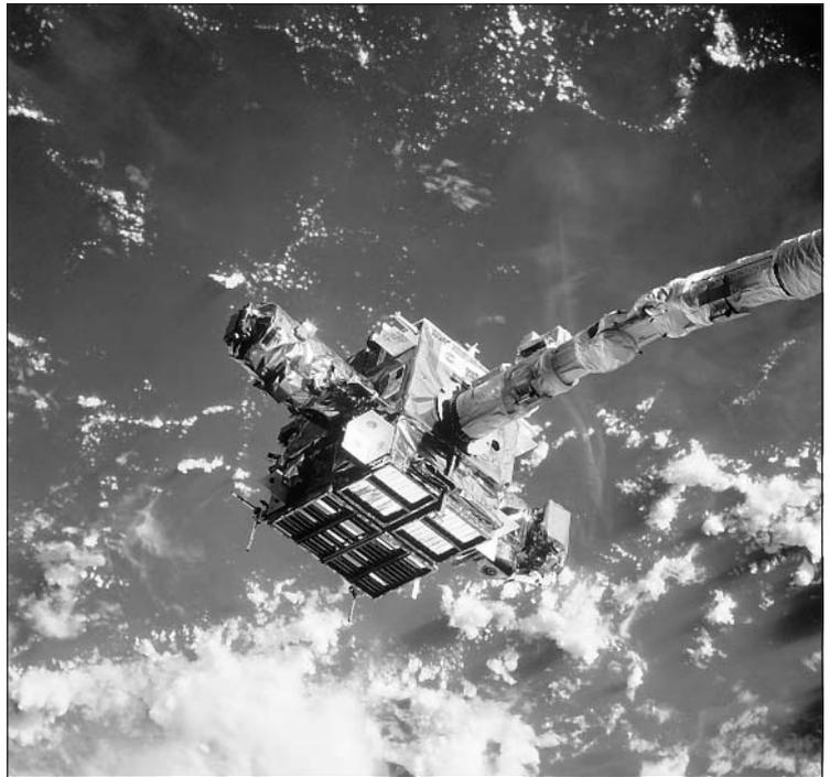
*The space shuttle deploys a satellite by means of a robotic arm. (NASA)*
