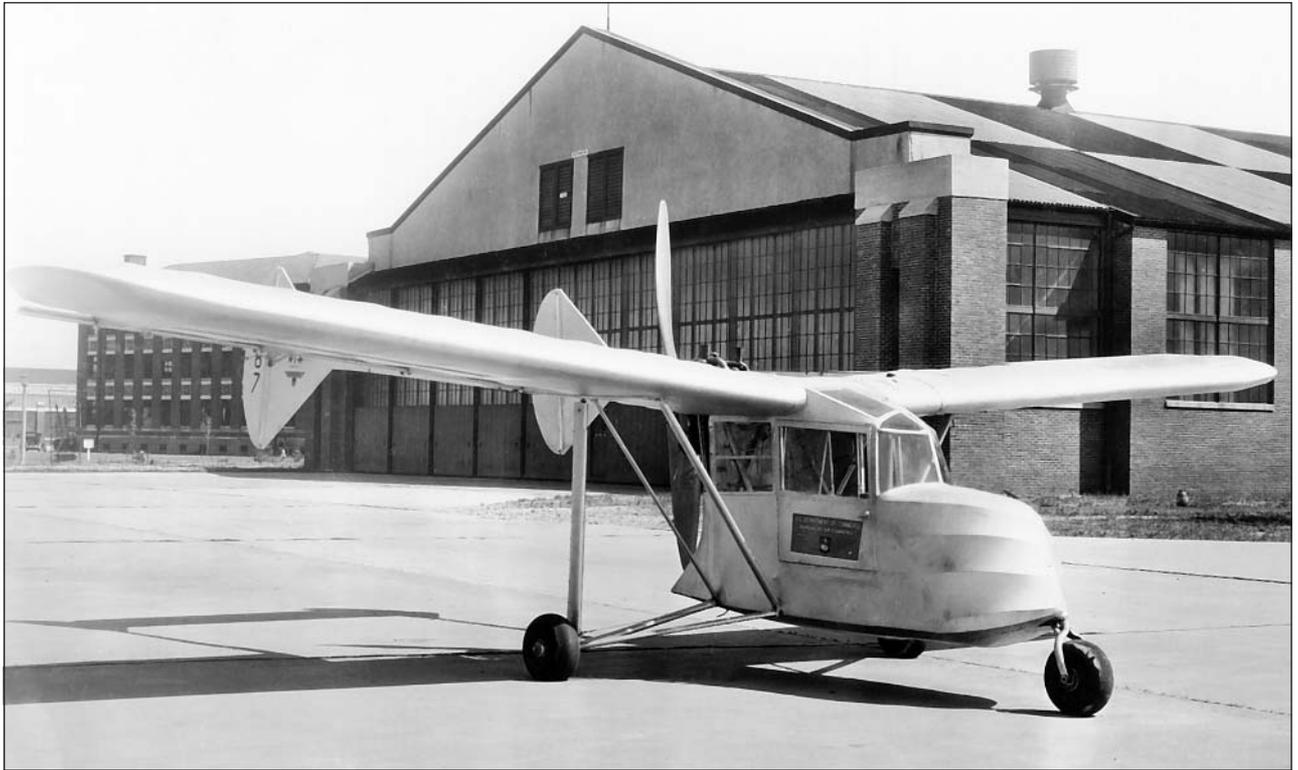
*Some experimental aircraft begin as homebuilt inventions to test new designs, such as Fred Weick's homebuilt 1934 W-1A, which experimented with the use of tricycle landing gear. (NASA)*
